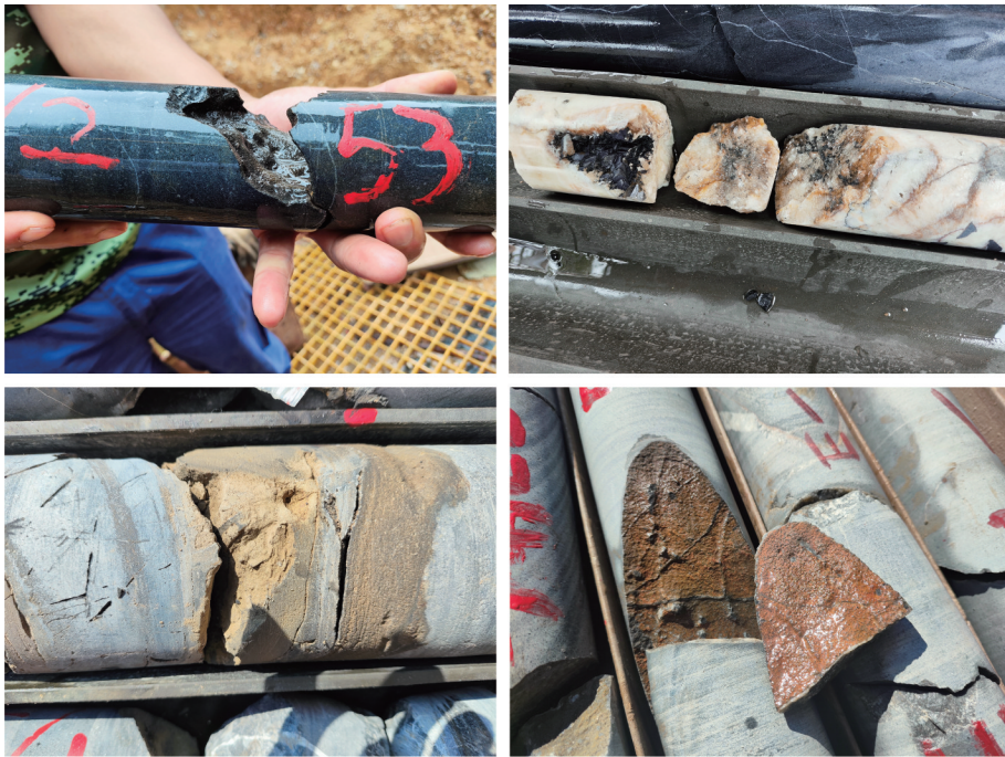
图2 多种岩溶裂隙 Fig.2 Various karst fissures
