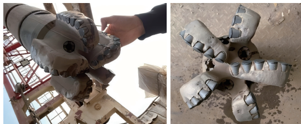
图 14 进尺 460.58 m 后的 PDC 钻头 Fig.14 PDC bit after footage of 460.58m
