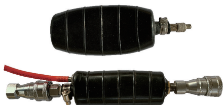
图3 基于DN50堵水气囊改造的密封气囊 Fig.3 Sealing airbag modified based on DN50 water-blocking airbag
