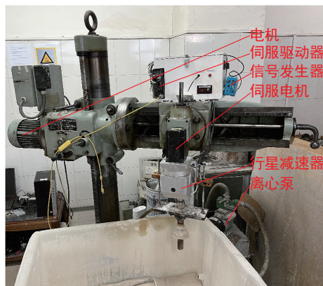
Fig.1 Servo feed micro-drilling test rig
