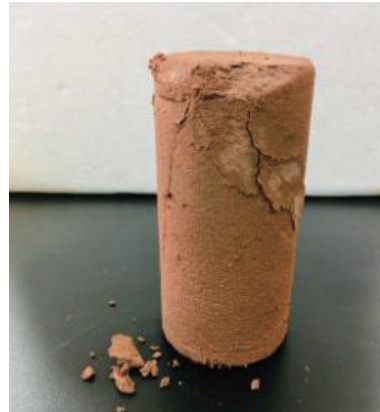
图 6 经 20 次冻融循环后饱和度 100% 红砂岩试样 Fig.6 Red sandstone sample with 100% saturation after 20 freeze-thaw cycles
