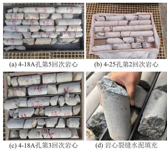
图 7 水平孔长距离取心照片 Fig.7 Long-distance coring photo of the horizontal well
