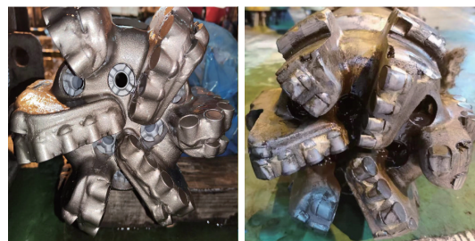
图5 HP636MI钻头的磨损情况 Fig.5 Wear of HP636MI
