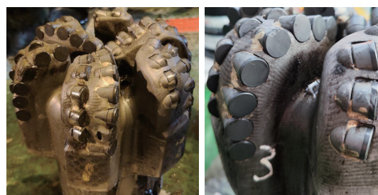
图11 旋转齿钻头磨损情况 Fig.11 Wear of bits equipped with rotating cutters
