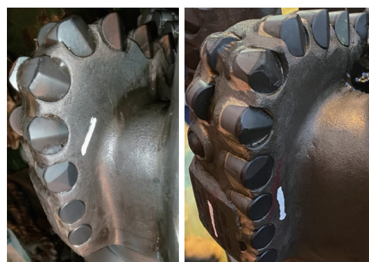
图12 斧形齿钻头磨损情况 Fig.12 Wear of drill bits equipped with axe-shaped cutters
