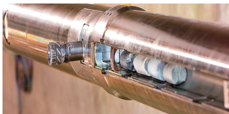
图4 Xaminer井壁取心工具 Fig.4 Xaminer sidewall coring tool
