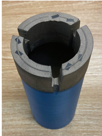
图4 烧结制备的钻头 Fig.4 Sintered drill bit
